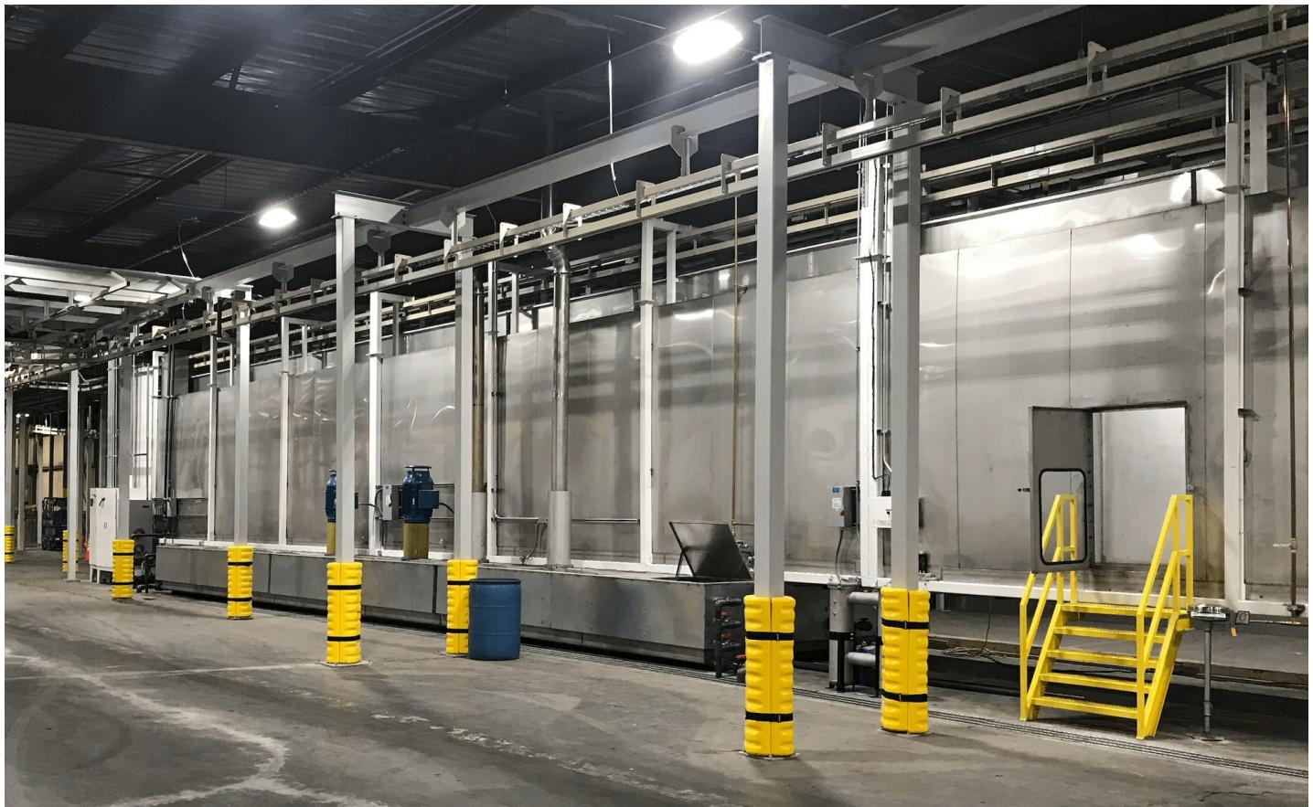
The integrity of the paint finishing process begins with pre-treatment. It is the first step in the finishing line, and it's critical to the outcome of the final paint quality. Chemical spray stages clean and coat the metal substrate as preparation for paint. Paint adhesion depends on a clean and thoroughly prepared substrate. Spray Tech pre-treatment washers save energy and lower operating costs
