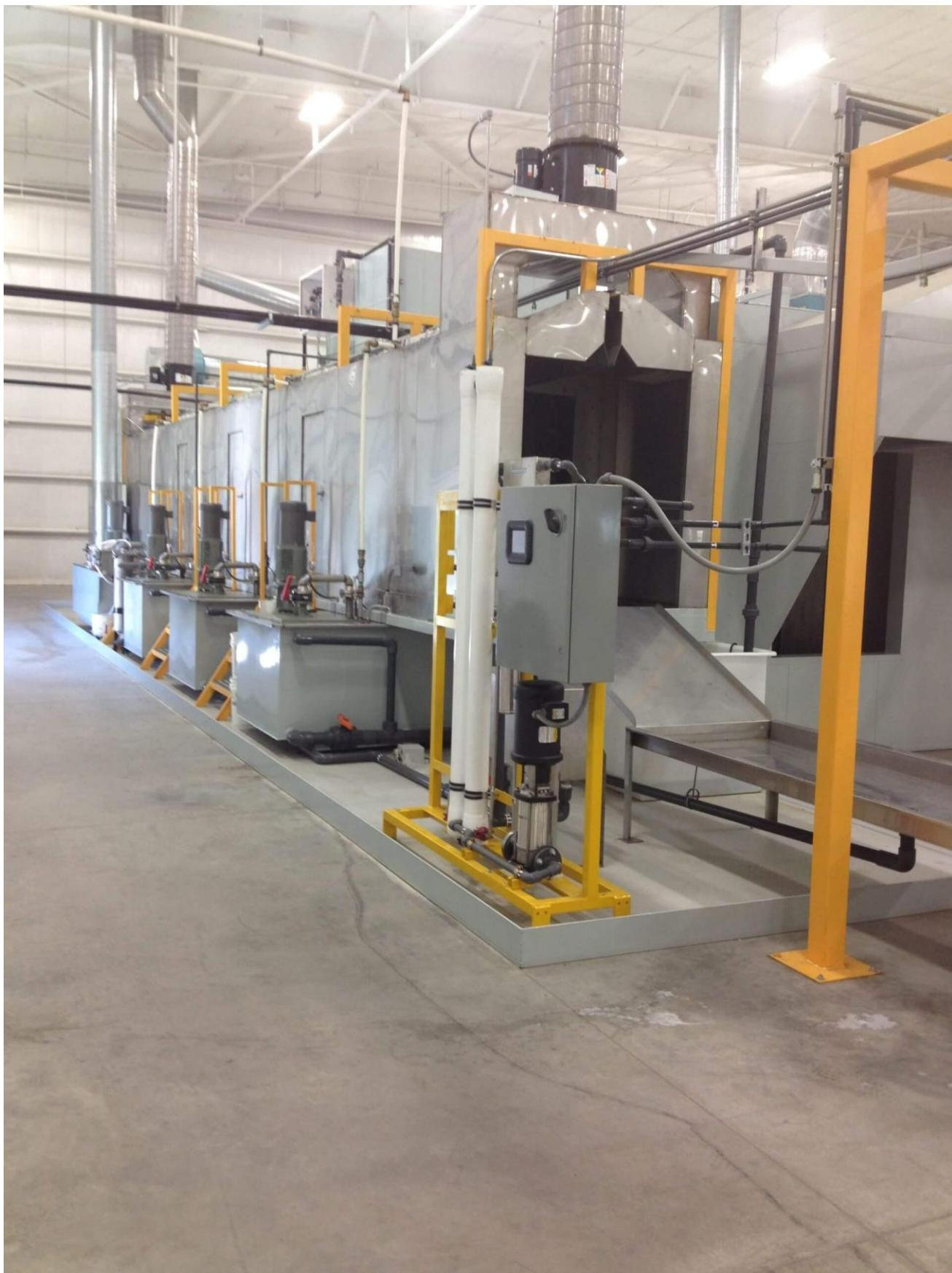
**Product Overview:** Spray Tech automated washers are efficient and consume less energy. Key design features include safe maintenance access, quick installation, and long service life. Spray Tech uses only best-in-class components. We select components for long service life, and we choose suppliers that offer local support. Every pre-treatment system meets chemical supplier specifications. Stage times, temperatures and material specifications are strictly adhered to.
