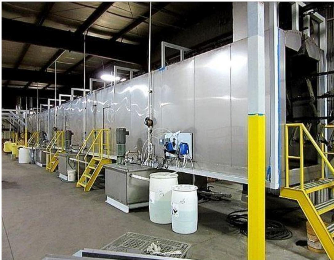
Operating pre-treatment washers can be costly. Spray Tech helps to lower operating costs through design. Using high efficiency components and added control features keep costs down. Our engineering focus is on lowering energy costs and reducing maintenance expenses through automated control features. PLCs control ancillary processes, such as blow-off and reverse osmosis systems, to minimize operating costs.
